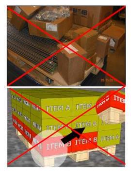
Stacking pallets is only allowed when it is 100% guaranteed that the goods and the delivered packaging will not be damaged.
